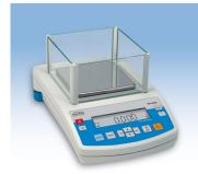
Balances series PS are equipped with 12 key front panel and LCD backlit display. Pan dimension is this series is 195×195 or 128×128 mm with a glass shield over the weighing pan which protects the load against possible breeze. Each balance has RS 232 and additional display outputs as standard.
